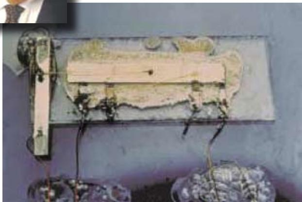
FIRST INTEGRATED CIRCUIT: Jack S. Kilby, *IL A '47*, inset, invented the integrated circuit at Texas Instruments in 1958. Comprised of only a transistor and other components on a slice of germanium, Kilby's invention, 7/16-by-1/16-inches in size, revolutionized the electronics industry.
