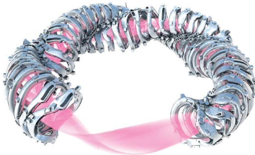
Left: Zap Energy's Z-pinch reactor does not rely on magnets to stabilize its plasma. Instead, it uses shear created by different layers of plasma moving at different speeds to maintain control. Credit: Zap Energy.
