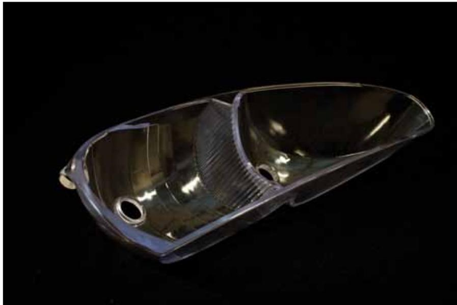
Headlamp casings are among the auto parts now being developed for the industry with the aid of 3D printing. Photos: 3D Systems.
