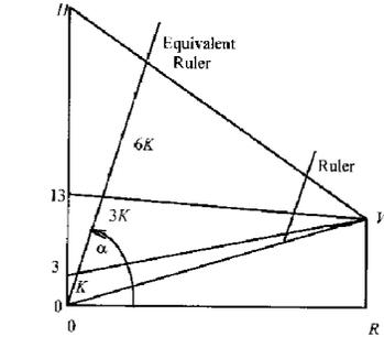
height of the viewer,  $R$  be the distance from bridge to viewer,  $\alpha$  be the angle of the ruler, and  $K$  be the proportionality factor for the ruler. Equations for the sightings of the heights of 3, 13, and  $H$  then are:
