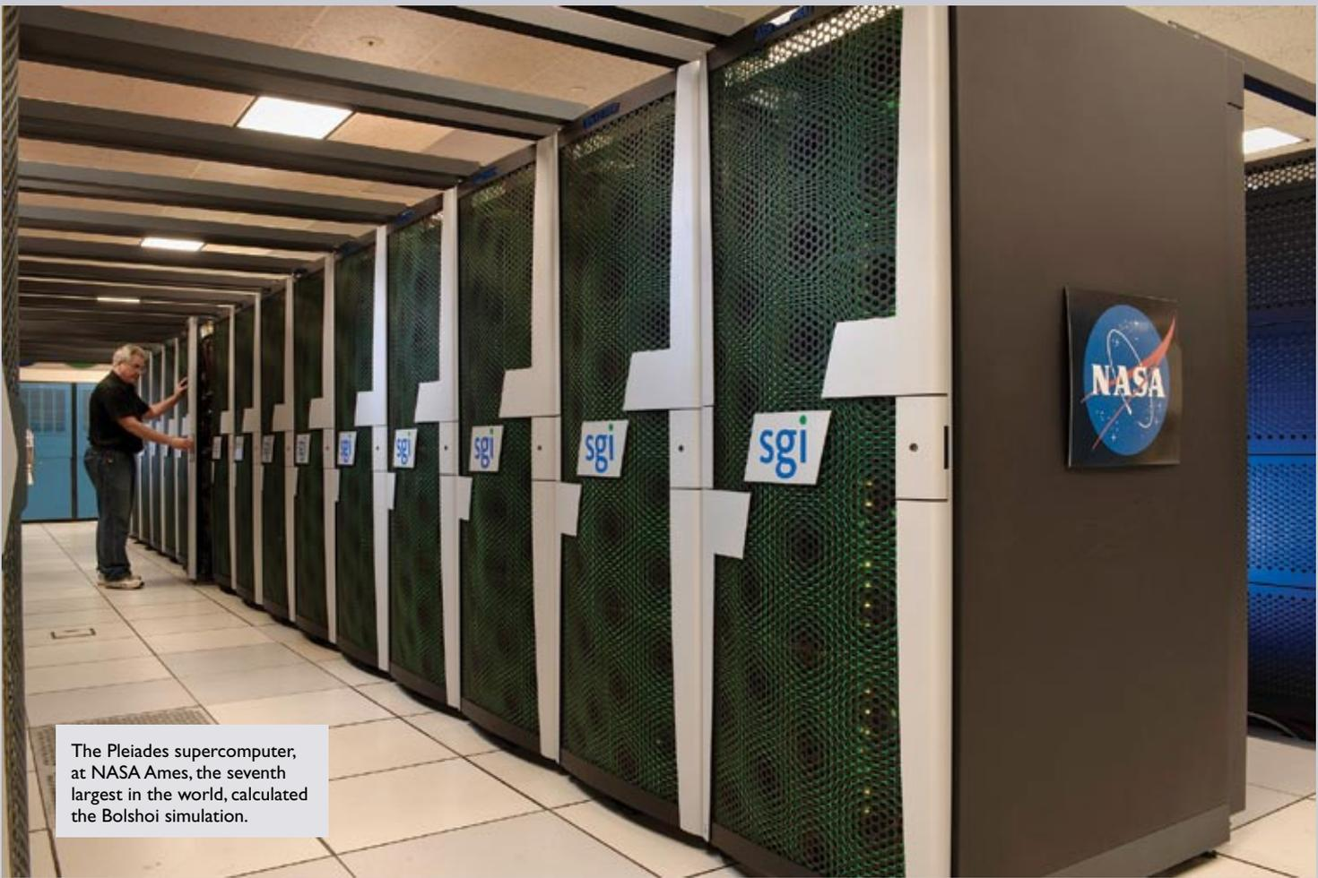
The Pleiades supercomputer, at NASA Ames, the seventh largest in the world, calculated the Bolshoi simulation.
