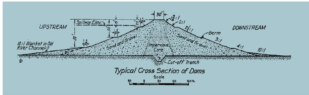
Diagram of the flood-control dams of the Miami Conservancy District shows their squat, triangular cross section. Each of the five dams, made of compacted earth, was topped by a roadway. Berms (shoulders or ledges) were provided at each change in slope to break the flow of rainwater down the faces of the dams as well as to function as roadways for inspection or maintenance.
