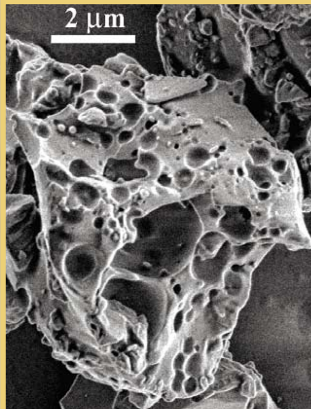
Lunar dust is full of tiny holes and is jagged like little burrs, making it uniquely abrasive and giving it a large surface area for its mass—characteristics that also give it bizarre properties that must be reckoned with by any astronauts returning to the Moon.
