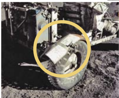
Lunar rover wheels stirred up so much dust (above) that makeshift dust fenders had to be added (left).
